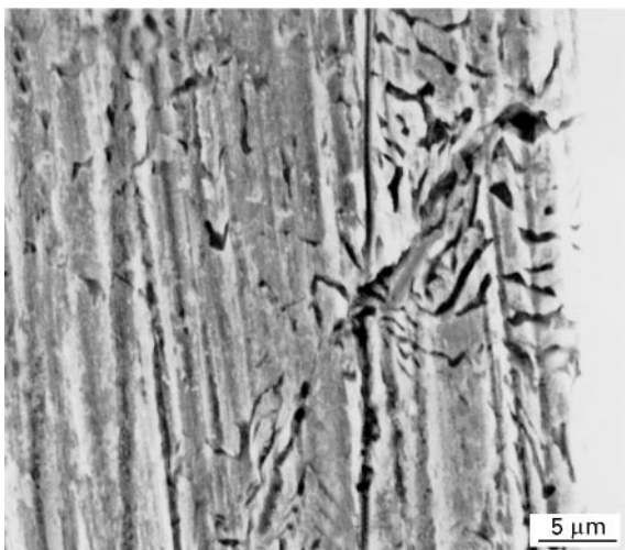
Figure 9 SCC initiation at the edge for specimen A after a total exposure of 15 h to distilled water at stress.
